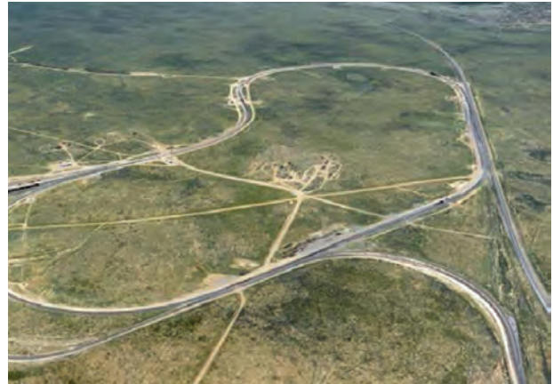
Figure 4. FAST's 4.3 km. High Tonnage Loop with three 340-to 400-meter curves and three full-scale bridges.
