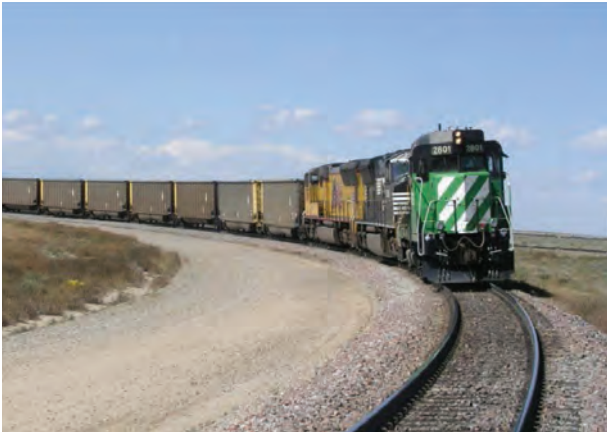
Figure 3. FAST's 16,000-tonne train equipped with 110 wagons with 35.3-metric-tonne axle loads.
