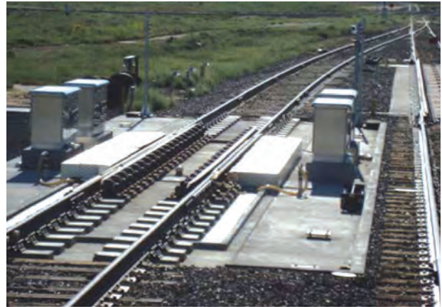
Figure 2. An automated Cracked Wheel Detection System under evaluation at TTC.
