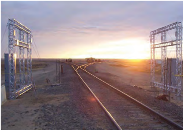
Figure 1. A machine vision inspection system, one of many defect-detection technologies being tested at TTC.
